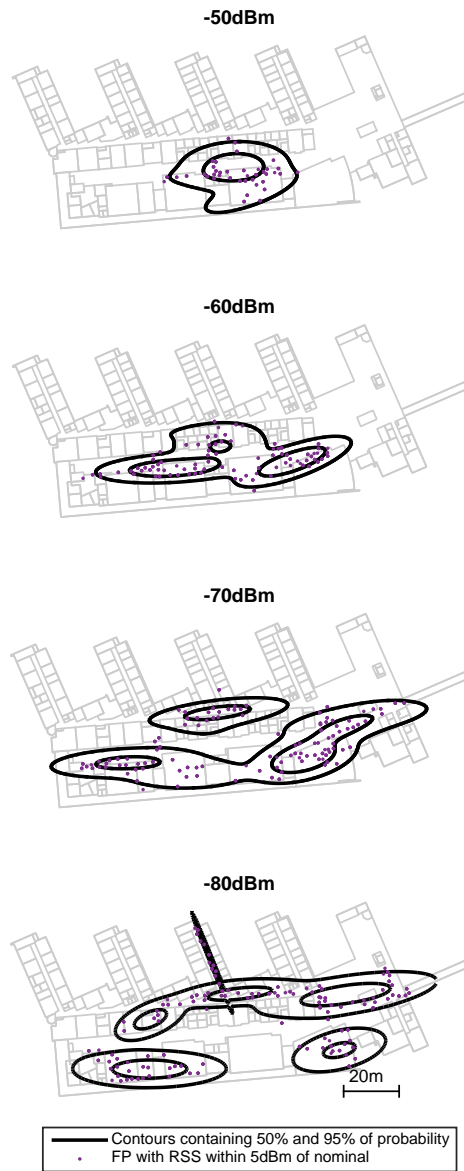
Figure 3: Conditional pdfs of the 2D positions when conditioning with RSS values and floor. For this building we had data from 4 floors. The conditioned contours show how the probability of the conditioned GMM is concentrated on the areas where the learning data was.
